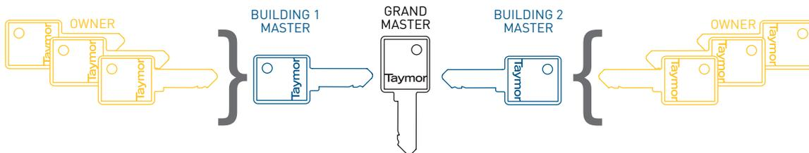
**CONSTRUCTION KEYING (CK)** allows the contractor of a project full access during the construction period. Once the owner's key is inserted, operation by the initial construction key is permanently disabled.
