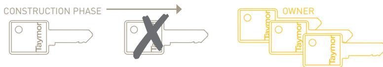
**DOUBLE KNOCKOUT CONSTRUCTION KEYING (CKRK)** adds a realtor key between the construction key and the owner key, which essentially allows a real estate professional to get temporary access until final handover to the buyer occurs. Once the owner's key is inserted, operation by the realtor key is permanently disabled.
